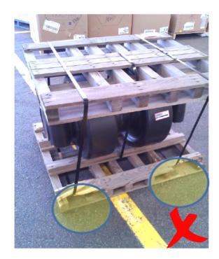
Applying straps or restraints over pallet boards without loaded weight can lift the board. Strapping should only be applied around boards if there is sufficient weight on the board to negate the force of the strapping.
