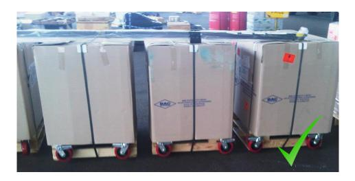
The above example highlights how to effectively limit movement from items supplied on wheels. These items must be stabilised for transport and the use of pallets underneath loads, with applied straps under the under bearers, is a perfect example on how to limit movement for safe transport.
