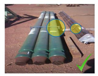
Example: Bundles are properly secured for transit Heavy steel or metal strapping/banding is required as in the examples here. It is also preferred that bundles have bearers strapped to enable forklift handling from underneath.
