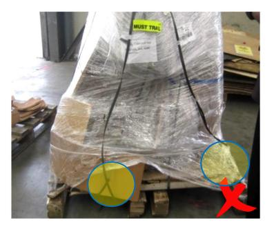
Example: Poorly strapped goods. Strapping has loosened in transit.
