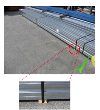
Example: Poorly packaged lengths for transit. Multiple lengths must be bundled tightly to prevent movement during transit. Bundles of steel require metal banding/ strapping for proper support.
