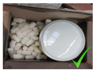
Example: Internal packing sufficient. Polystyrene foam assists to hold this drum in the carton
