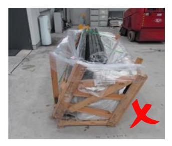
Example above: a poorly crated item. The contents are too heavy for the flimsy crate construction. The heavy items were not adequately restrained by the plastic straps, so movement has resulted in the crate collapsing.
